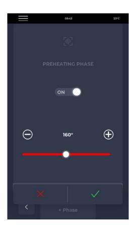
N.B. It is possible to set a preheating phase of the cooking chamber and its relative temperature.
