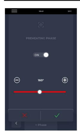
N.B. It is possible to set a preheating phase of the cooking chamber and its relative temperature.
