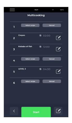
After confirming the general settings of the programme, the levels in which to insert the recipes or alternatively a manual programme will appear on the display.
